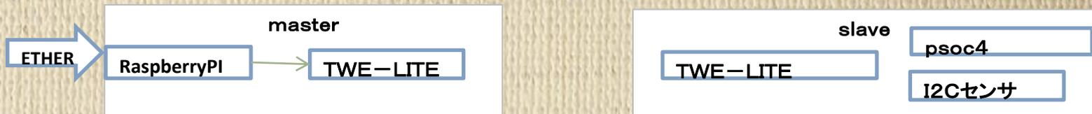
3)RaspberryPI→TWE-LITE.....TWE-LITE→Serial to I2C
